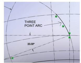
9. Now sketch a Tangent Arc. This arc will represent the bottom edge of one of the gear teeth. Start this arc on the bottom end point of the 3 Point Arc, sketched in the step above, to the Root Diameter circle. This arc needs to be perpendicular to the Root Diameter circle. Refer to the image nearby.
